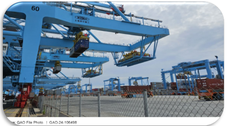
Figure 111. Semi-automated double trolley cranes load containers onto automated guided vehicles
