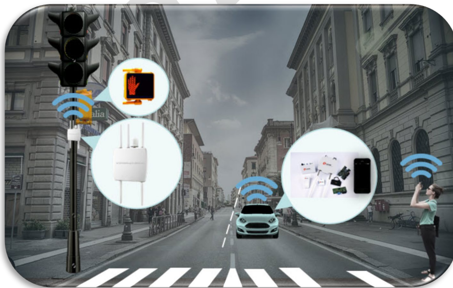
Figure 89. PedSafe: Pedestrian and Bicycle Collision Avoidance System by FDOT utilizing Connected Vehicle technology.
