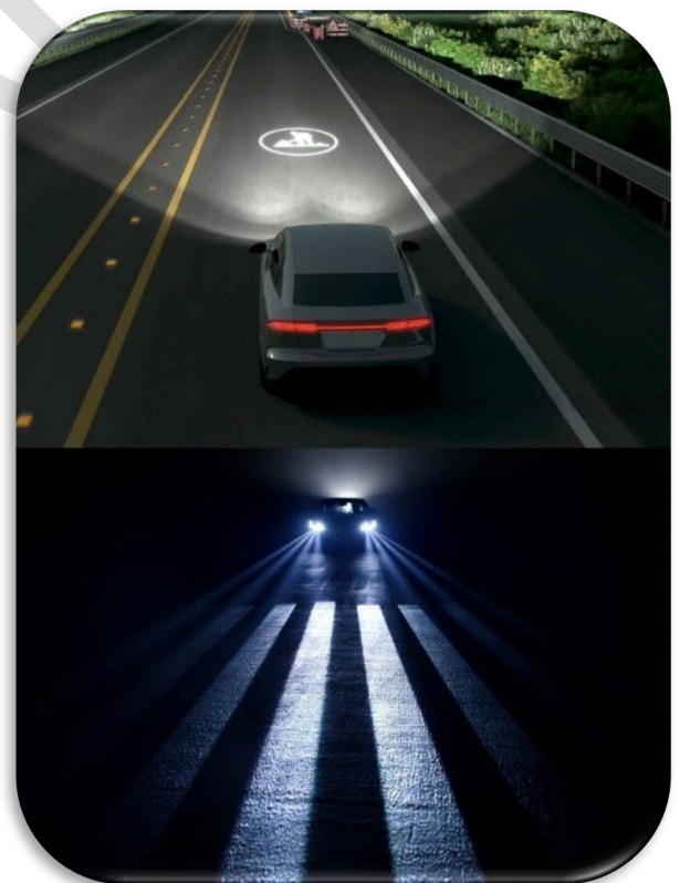
Figure 93. HD lighting system technology projects street signs on road.
